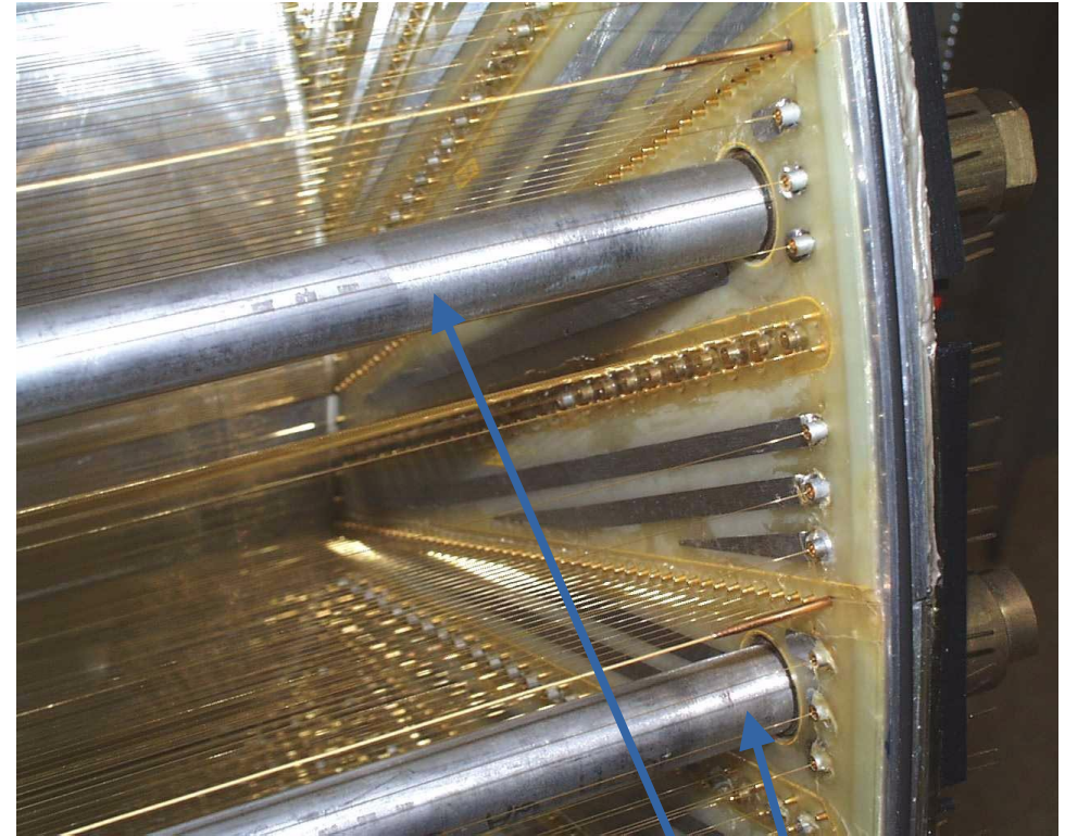
H1 Drift Chamber: ~15000 wires, 6 tons of force
